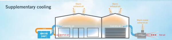
Climate Wizard used with an air cooling system to provide supplementary cooling.
