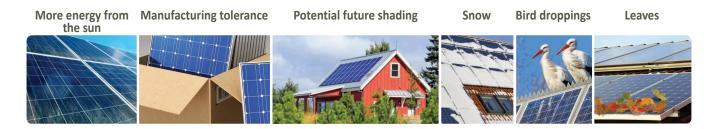
With traditional inverters, the weakest module reduces the performance of all modules.
