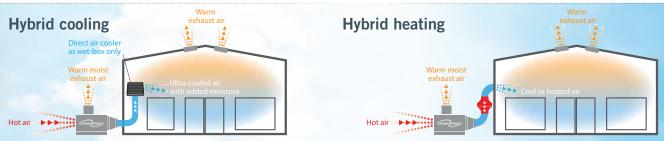
Climate Wizard is combined with other complimentary devices, such as direct evaporative 'wet-boxes' or heating devices; such as elements, hot water coils, gas-fired exchangers to successfully resolve a variety of heat load and comfort challenges.
